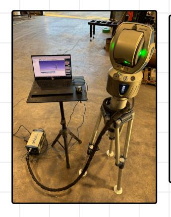
The FARO Laser Tracker is a highly precise, portable coordinate measuring machine that enhances our ability to build products, optimize processes, and deliver solutions with speed. The FARO Vantage laser tracking tool enhances the precision of our metrology services.
