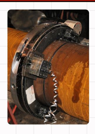
Bevel Tech Group, Inc. provides a variety of clamshell pipe cutting machines, ranging from 2" to 120", designed for hands-free operation. These innovative machines prioritize safety by keeping operators out of the hazard zone during cutting and beveling, delivering a ready-to-fit surface upon completion.
