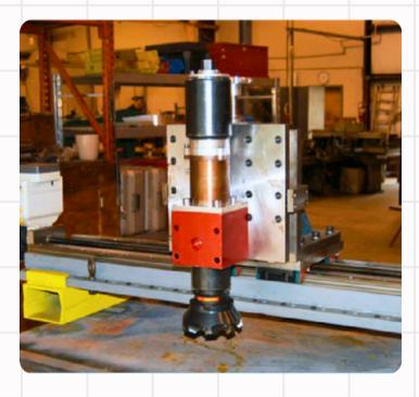
This 60" portable milling machine is ideal for milling pump and motor pads.
