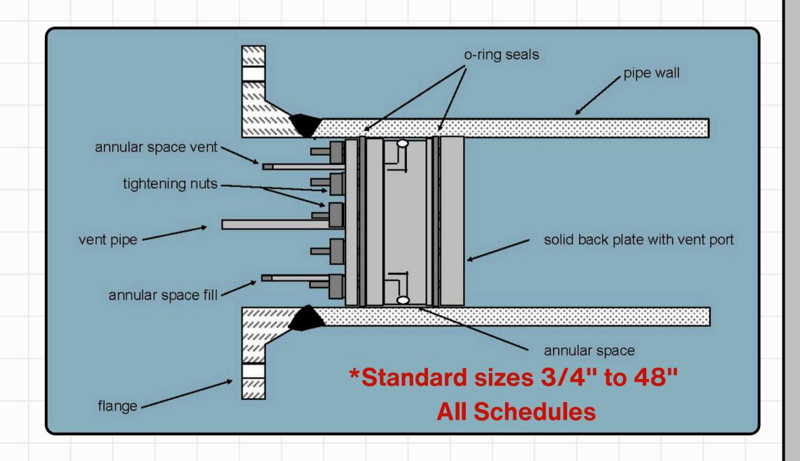
Bevel Tech Group's pipeline isolation tooling can positively isolate and monitor potentially explosive vapors while performing the hot work on the upstream line
