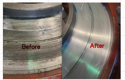
Our portable ID flange machines can resurface flanges from 4 ft. to 18 ft.
